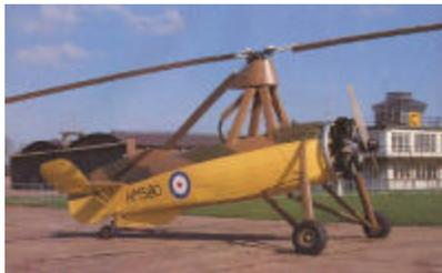
This strange aircraft was really a predecessor to modern day helicopters. The difference is ... the autogiro did not have an engine turning the rotor blades. They were free-spinning.
