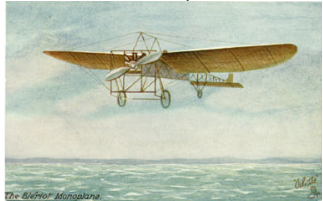
Designed by Louis Blériot this was a light and sleek monoplane constructed of oak and poplar.
